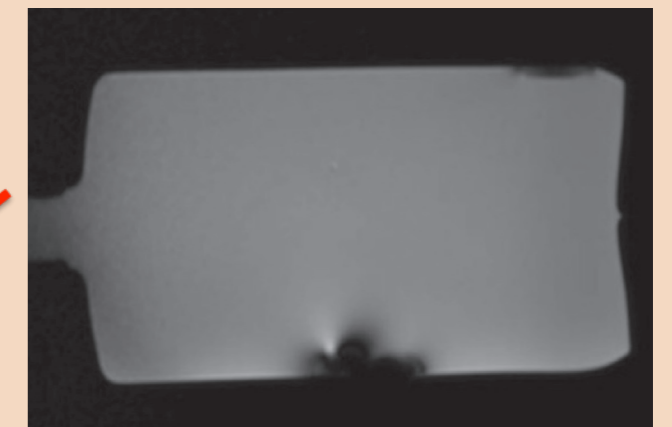
MRI image of artefact caused by the RF tag in the sheet
