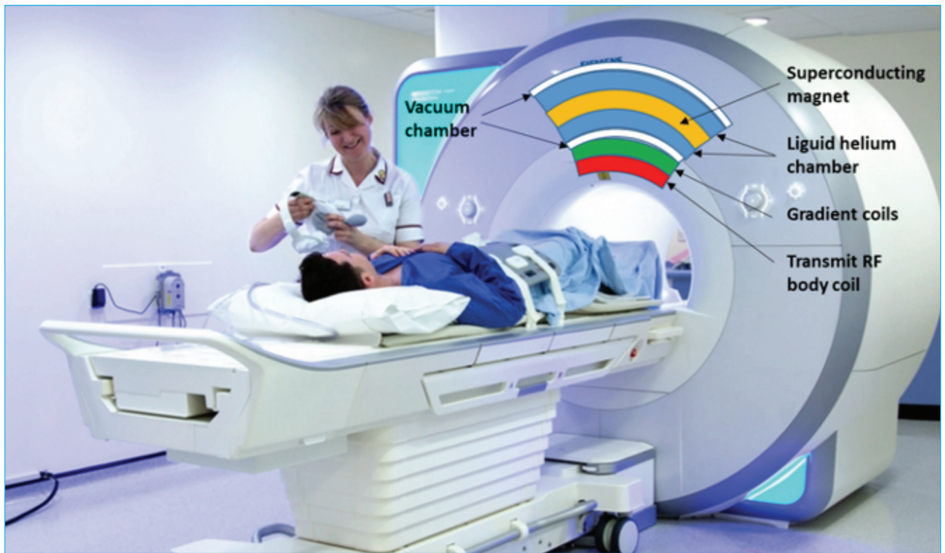
◆ Figure 1: Simplified diagram of the concentric arrangement of the coils in the MR scanner. (Courtesy of The Royal Marsden Hospital, London, UK).
