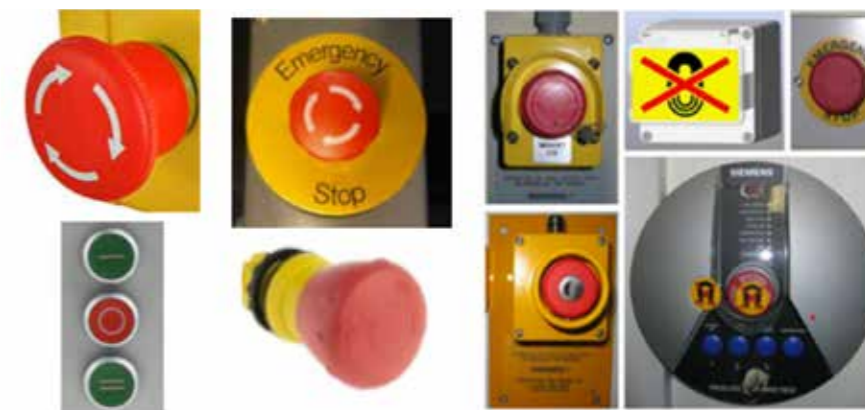
◆ Figure 3 Images showing the variety of emergency buttons that the fire teams may be faced with
