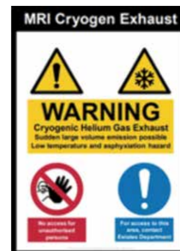
◆ Figure 4 Quench pipe warning notice
