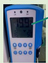
Mobile MRI units often use a portable oxygen monitoring system, Check if the batteries need to be replaced.
